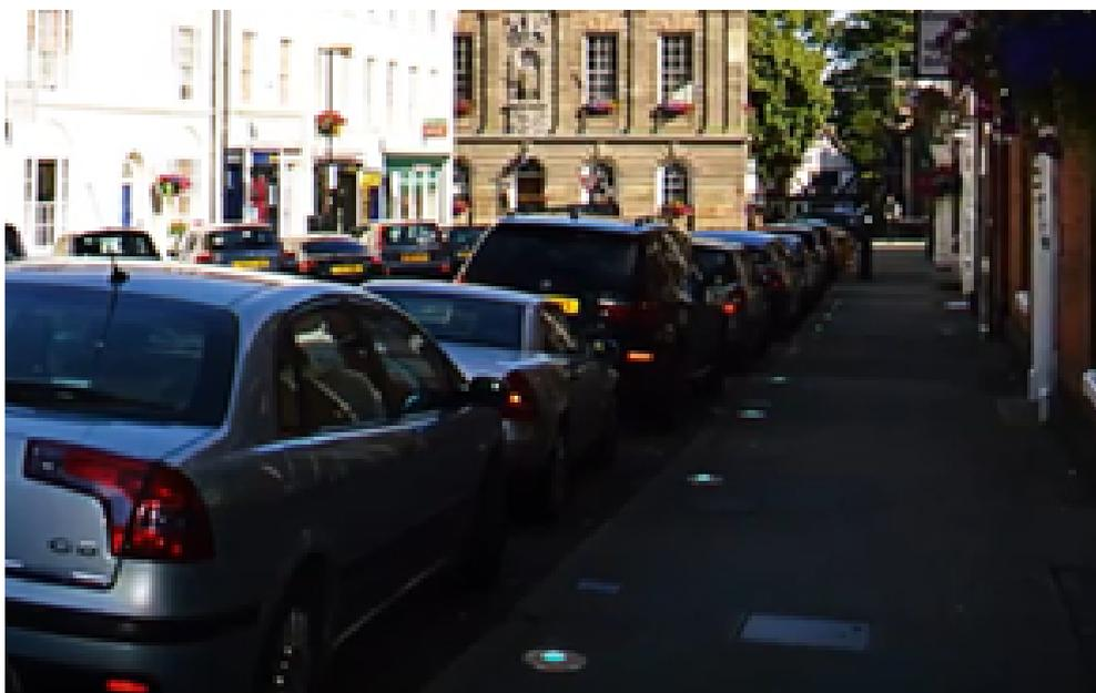
5.5.3. The Trojan system is made up of 'flush' connector placed at the front of the footway as can be seen the photo (small lights at the kerb edge)
